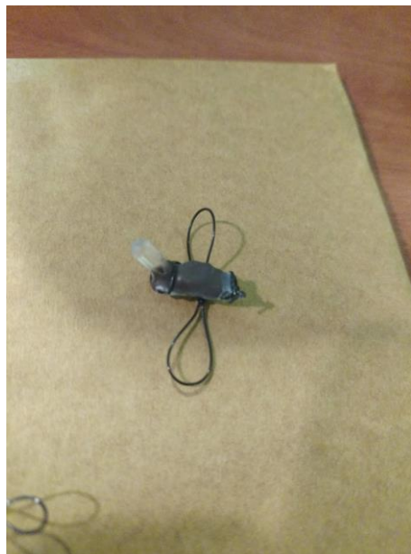
Light-level geocator ready to deploy on Cerulean Warbler by Clayton Delancey—June 2017
